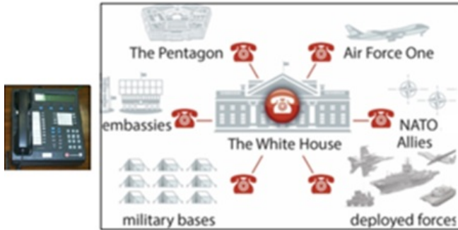
Fig. 12. Secure Terminal Equipment, STE; note slot in front for Crypto PC Card (left). The DRSN architecture (right).
