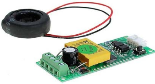
Figure 14. AC Power Sensing Device
