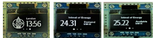
(a) (b) (c) Figure 13: OLED Screen Presentation for Node 2. (a) Local Time, (b) Power Demand, (c) Available Power
