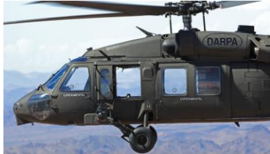
Fig. 5. Sikorsky’s Optionally Piloted Black Hawk aircraft demonstrating uninhabited resupply in 2022. When the MATRIX system is fully integrated on a UH-60M, this aircraft will closely resemble Sikorsky’s UH-60A Optionally Piloted Black Hawk in this image.
