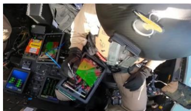
Fig. 6. Test pilots control an ALIAS/MATRIX-equipped UH-60A Black Hawk with a tablet interface during a test flight.
