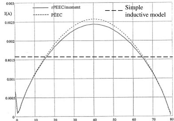
Figure 10-b. current distribution for  $L_1=L_2=\lambda/8$
