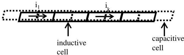
Figure 1. Conductor subdivision into inductive and capacitive cells
