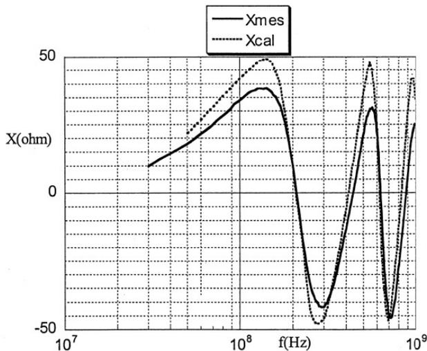
Figure 9-b. Imaginary part of the input impedance calculation/measurement
