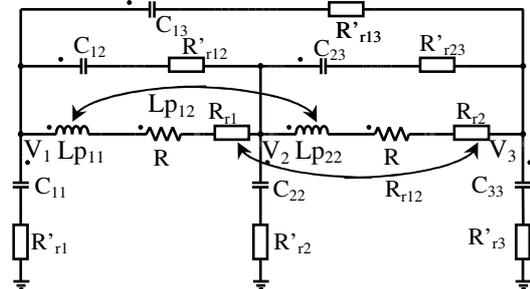
Figure 3. rPEEC equivalent circuit
