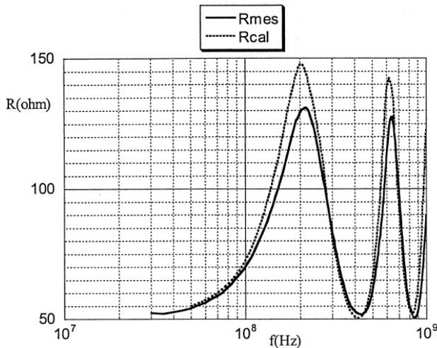
Figure 9-a. Real part of the input impedance calculation/measurement
