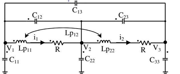
Figure 2. PEEC equivalent circuit
