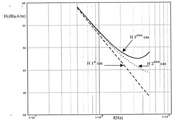
Figure 14. effect of retardation on magnetic field.
