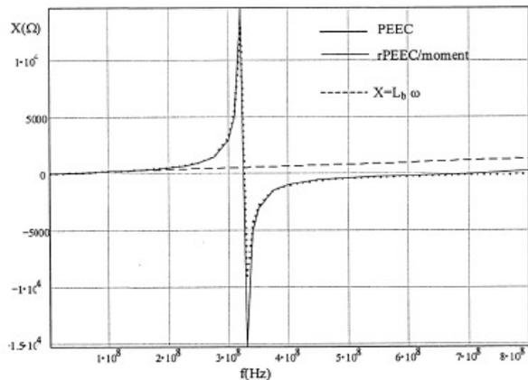
Figure 11. imaginary part of input impedance of a loop conductor
