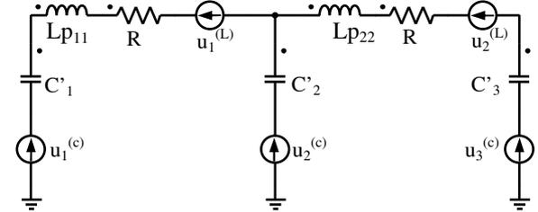
Figure 4. rPEEC model proposed by A. Ruehli.
