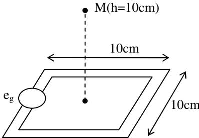
Figure 13. magnetic field radiated by a loop.
