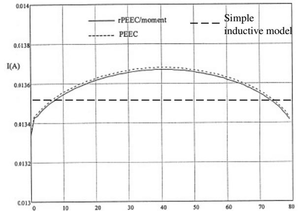
Figure 10-a. current distribution for  $L_1=L_2=\lambda/64$
