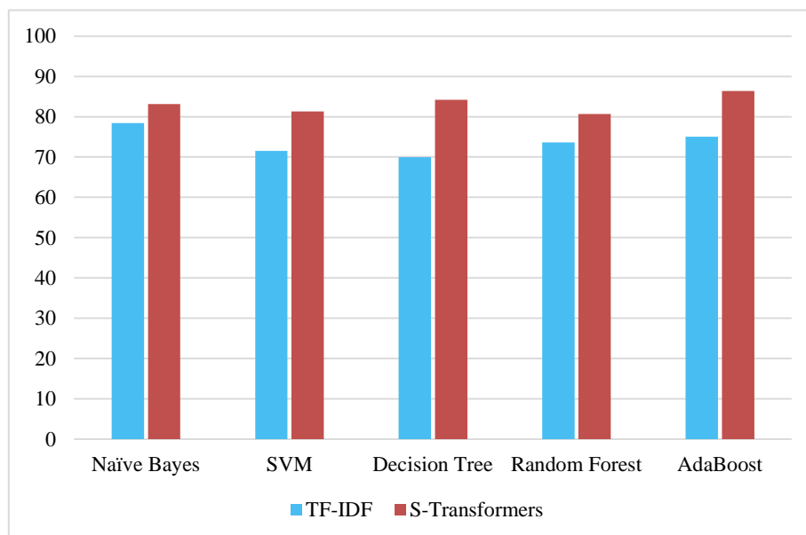
Figure 3. Accuracy Comparison of Diverse ML Models using TF-IDF and Sentence Transformer Encoding
